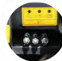
09 Centralized lubrication points
