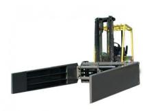
Multifunction clamp to load with full boxes, empty boxes, or to palletize several pallets together. Attach on FEM2 / FEM3 board. 3 versions available. Ask us.
