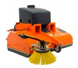
Mechanical sweeper to insert in wheelbarrow nails with side brush. With a width of the main brush of 1550mm and a waste tank. Easy to use and mount on forklift trucks.
