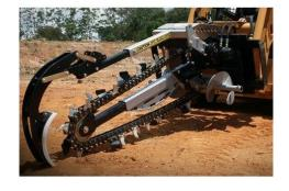
High performance trenchers with different types of chain, for the opening of ditches in all types of vegetable, mixed and compact terrains, even very hard or with roots.
