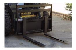
The Ty 1000 pallet carrier with load backing and guides for lateral displacement of the forks, is ideal for loading and transporting pallets safely for construction, industry, gardening, agriculture, livestock ...
